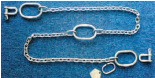
Pump lifting chains
